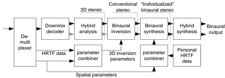
Figure 10: Binaural (re)synthesis using individual HRTFs based on a 3D-stereo downmix.
