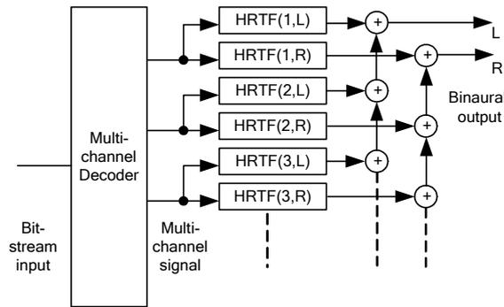
Figure 1: Decoding and binaural rendering of multi-channel signals.
