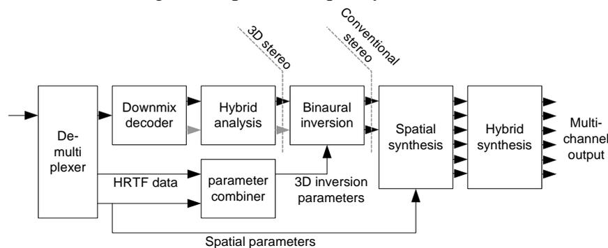
Figure 9: 3D decoder for loudspeaker playback.
