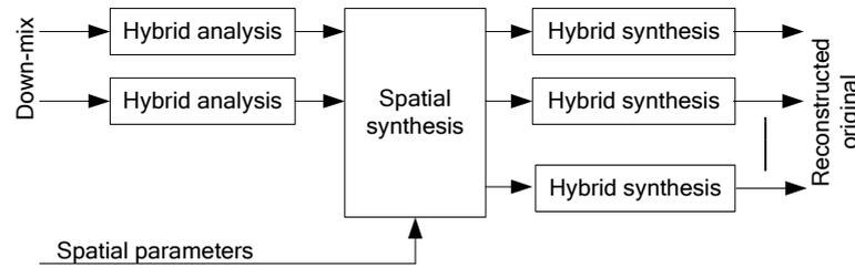
Figure 3: High level MPEG Surround decoder structure.
