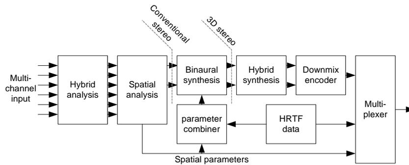
Figure 8: 3D encoder schematic
