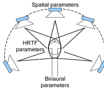
Figure 6: Binaural parameters result from spatial parameters and HRTF parameters
