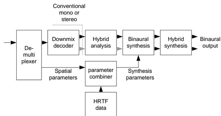
Figure 7: Binaural decoder schematic.
