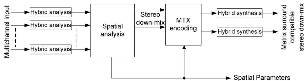
Figure 5: MPEG Surround encoder with post-processing for matrix surround (MTX) compatible downmix.
