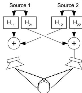
Figure 11: Crosstalk (dashed lines) and crosstalk cancellation filters ( $H_{xy}$ ) for 2 sound sources.
