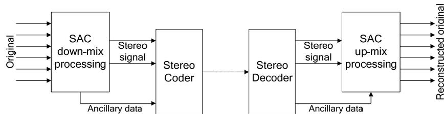
Figure 2: Typical SAC encoder/decoder chain.
